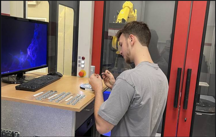
BLUE-LIGHT SCANNING ON THE ATOS SCANBOX
